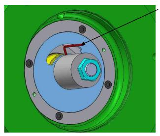
Use Allen key to tighten (fix) the threaded bolts that have been moistened with Loctite.
