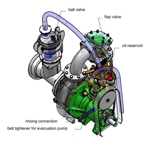
The **centrifugal pump** is not able to take in the medium (water or slurry) itself – this is done by the self-priming device.
