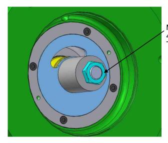
Mount the space-adjusting nut - mounting length 47.5  $\pm$  0.5mm. Tighten the nut by hand.
