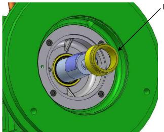
Press the mechanical seal on
